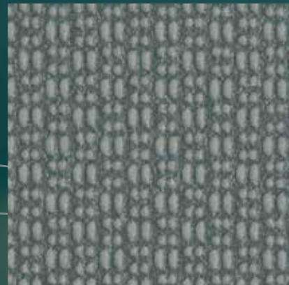
graboVaporex sheet underlays specially coated and patterned reinforced with fiberglass materials enable the safe installation of floor coverings on slightly moist or contaminated subfloors. Additionally Vaporex 40 has excellent sound insulating property.
